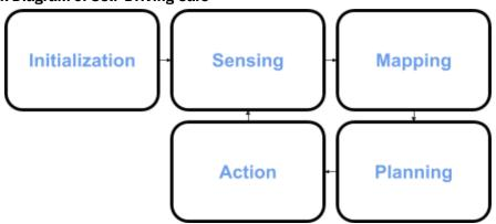
Initialization - Calibrating the robot and creating the datasets that are necessary to get the robot ready to drive
